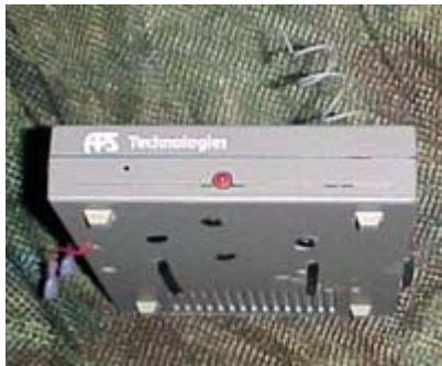
Front View. The red LED lights up when the unit is powered on and off and also when the unit has received a signal and is sending current through.
